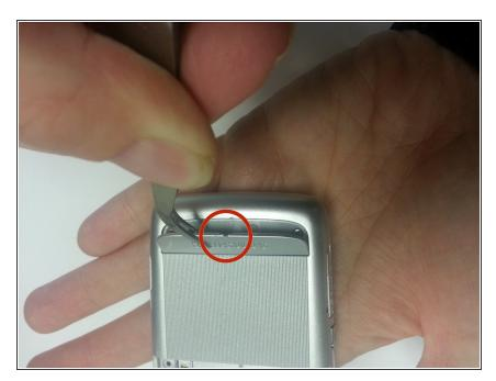
Gently insert a pair of tweezers under the Samsung logo on the bottom of the phone. Then unscrew the two .4 cm Phillips head screws underneath.
