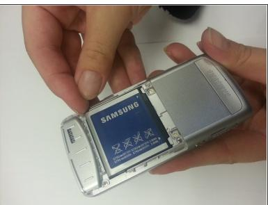
Using your finger, grasp the corner on either side of the battery and pull up.
