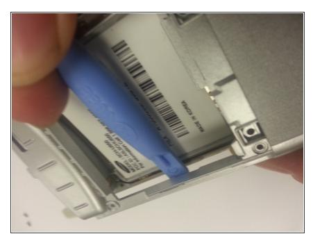
Gently insert the plastic opening tool into the seam where the battery was located. Work the opening tool around until the back cover comes off. Make sure to be careful of the side buttons that pop off.
