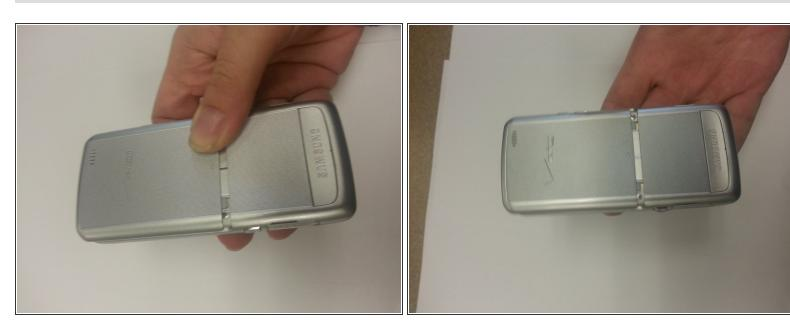
Using your thumb(s) slide the battery cover up to remove it.
