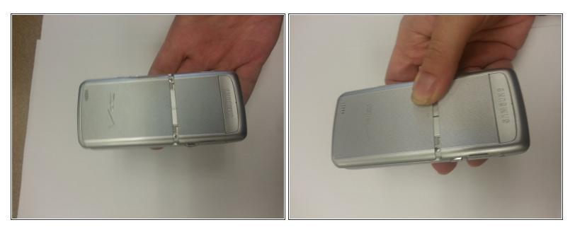
• Using your thumb, slide the cover away from the device, and then place the cover to the side.
