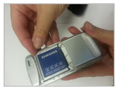
• Grip the corner of the battery on either the left or right side with your fingers and lift it up to remove it.
