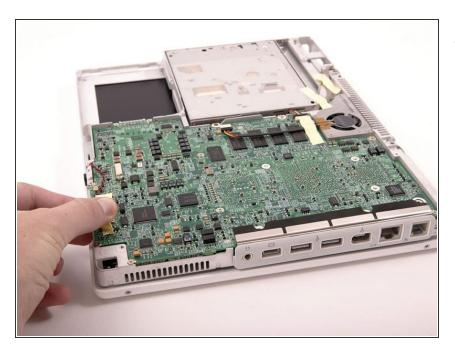
Turn the computer over and disconnect the orange hard drive cable, removing tape as necessary.
