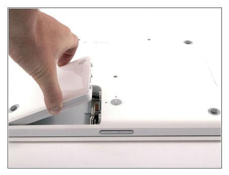
Lift the battery out of the computer.
