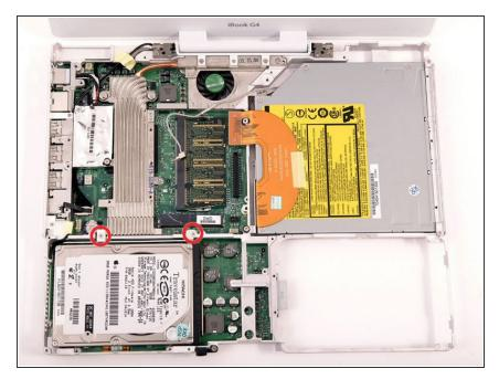
Remove the two Phillips screws securing the hard drive to the metal framework.
