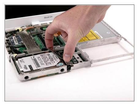
Lift the metal restraining bracket from the hard drive and place it aside.
