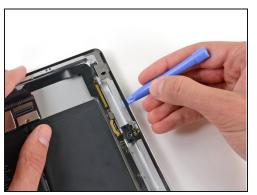
Be mindful of the front facing camera when sliding the plastic opening tool along the top edge of the iPad.
