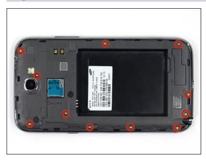
Remove the eleven 4.0 mm Phillips #00 screws securing the midframe to the display assembly.
