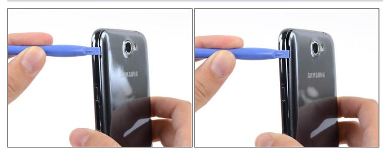
• Pry with a plastic opening tool, or your fingernail, in the divot to the left of the rearfacing camera, near the power button.
