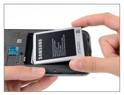
• Remove the battery from the midframe.
