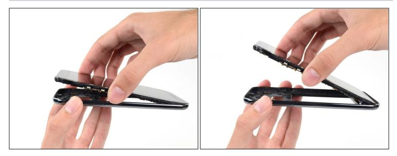
• Lift the display assembly out of the midframe.
