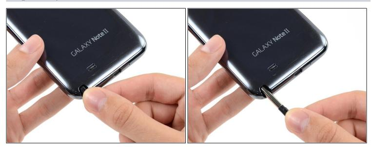
• Grasp the end of the stylus and remove it from its slot in the midframe.
