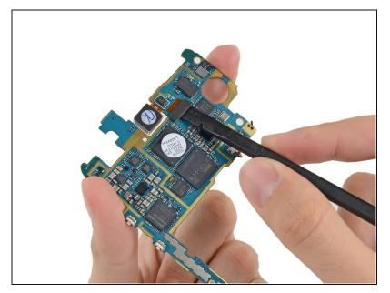
• Use a spudger to disconnect the rear-facing camera assembly cable connector.
