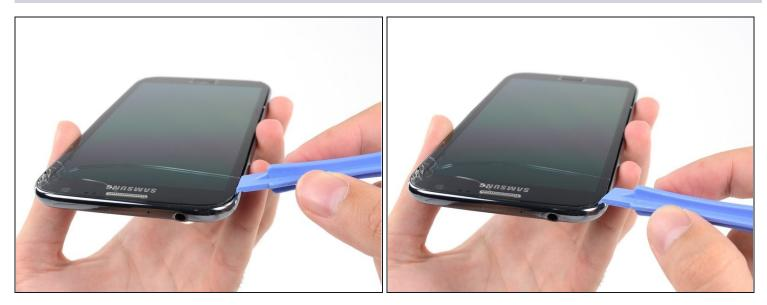
• Carefully pry around the corner with a plastic opening tool.
