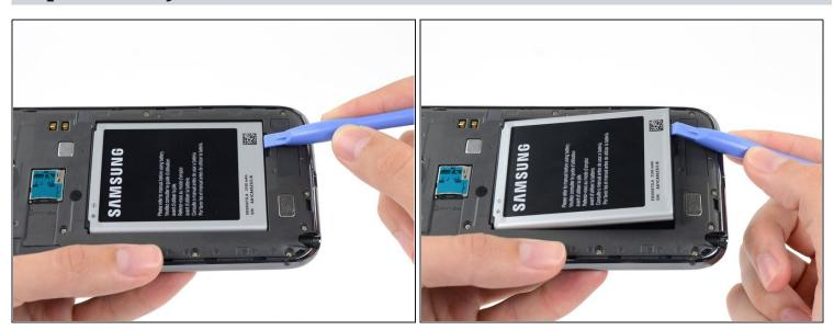
• Insert a plastic opening tool, or your finger, into the notch of the battery compartment and lift the battery upward.
