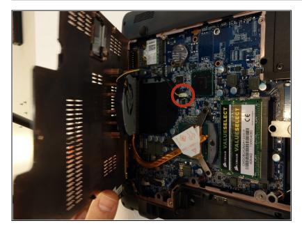
• Since the ventillator is mounted under the cover, its power supply cable must first be disconnected so that the cover can then be completely removed.
