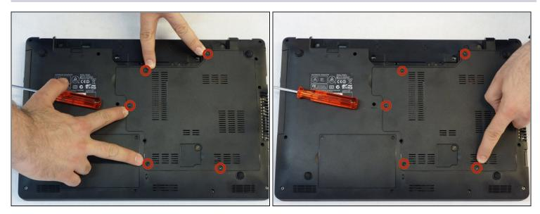
• Using a Philips #1 screwdriver, unscrew the 5 screws securing the cover.
