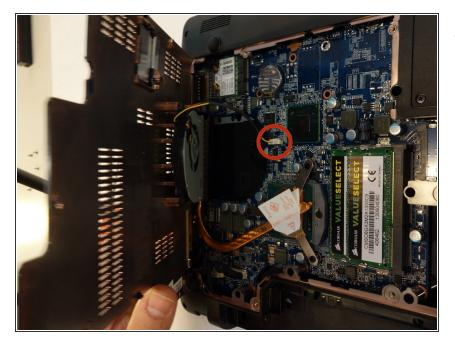
Since the ventillator is mounted under the cover, its power supply cable must first be disconnected so that the cover can then be completely removed.
