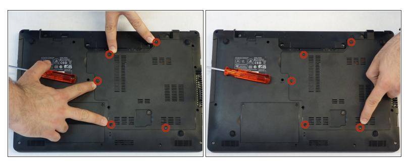
• Using a Philips #1 screwdriver, unscrew the 5 screws securing the cover.
