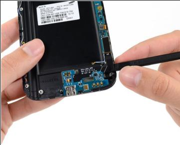
• Push the flat end of a spudger under the USB board to separate it from the display assembly.
