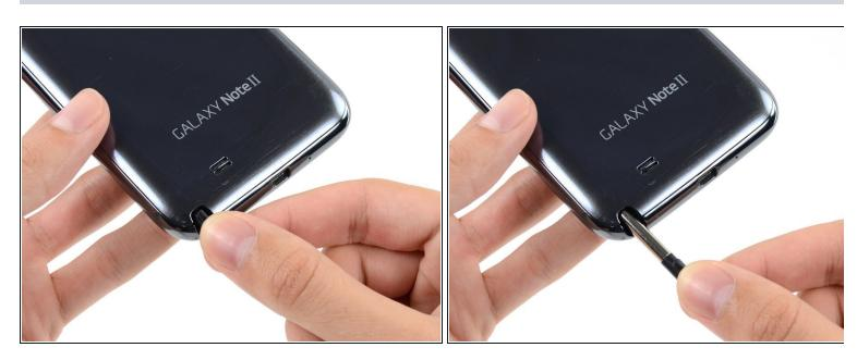
Grasp the end of the stylus and remove it from its slot in the midframe.
