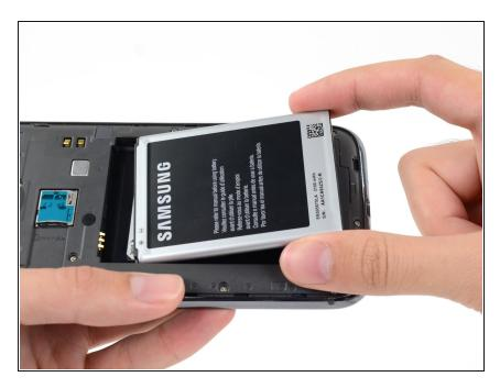
Remove the battery from the midframe.
