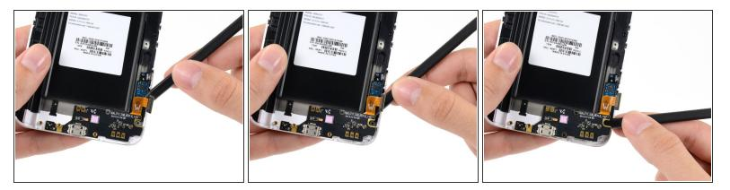
• Push the flat end of a spudger under the USB board to separate it from the display assembly.
