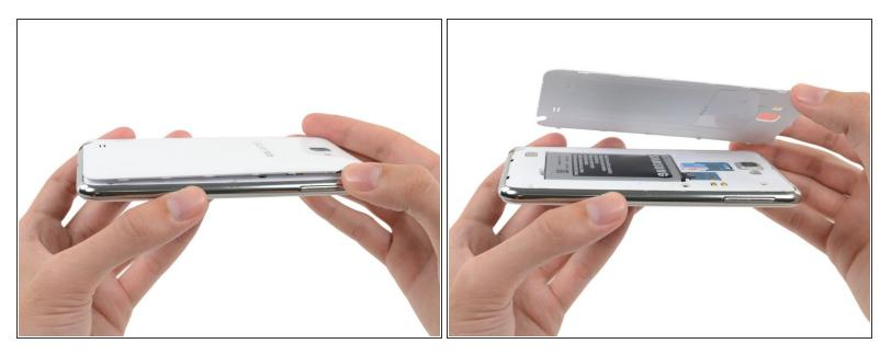
• Lift and remove the rear case from the phone.
