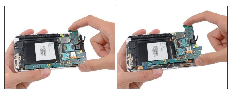
• Remove the motherboard assembly from the display assembly.
