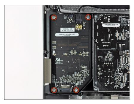
Remove the four T10 Torx screws securing the LED driver board to the outer case.
