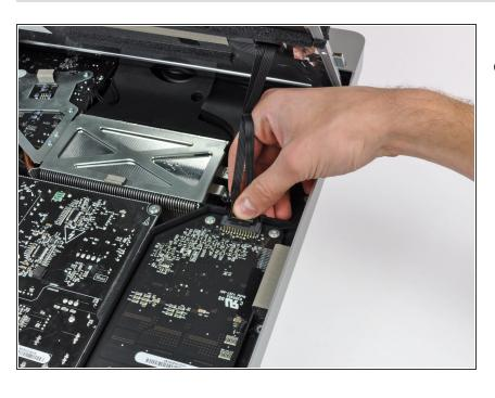
Rotate the display out of the outer case enough to disconnect the LED backlight power cable from the LED driver board.
