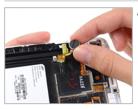
Remove the vibrator from the display assembly.
