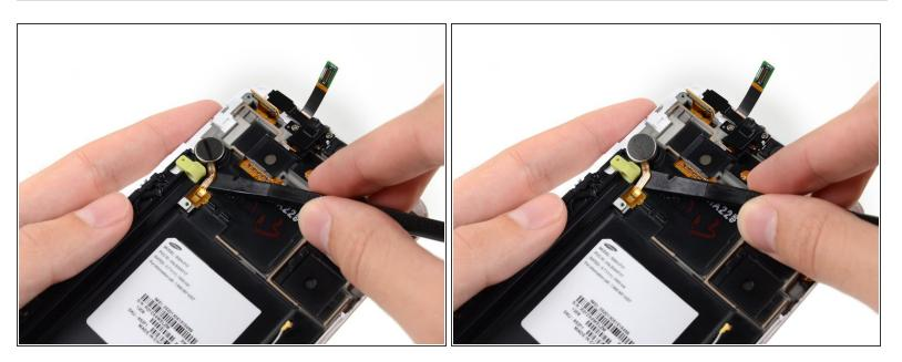
Insert the flat end of a spudger under the vibrator connector cable and pry it up from the adhesive.
