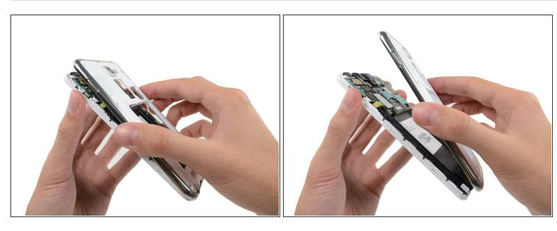
Remove the midframe from the display assembly.
