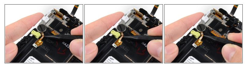
Insert the tip of a spudger under the vibrator connector cable near the contacts then slide it toward the vibrator itself.
