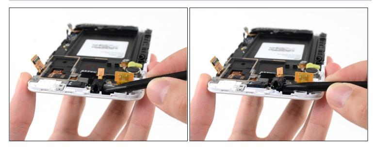
• Use the tip of a spudger to pry the headphone jack/earpiece speaker assembly out of its recess in the display assembly.
