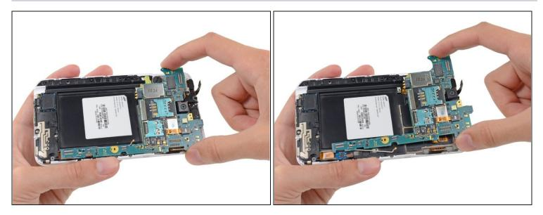
• Remove the motherboard assembly from the display assembly.
