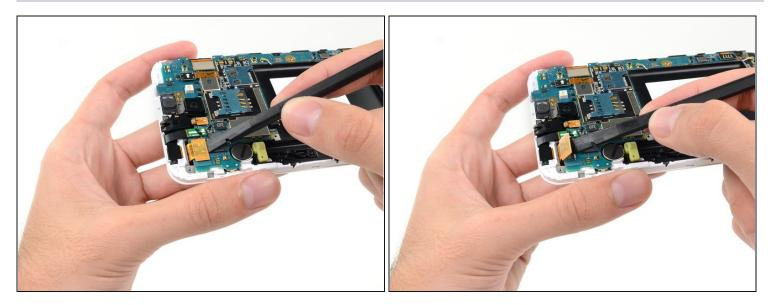
• Use the flat end of a spudger to carefully disconnect the display cable connector.
