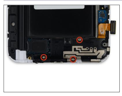
Remove the three 3 mm Phillips #00 screws securing the speaker enclosure to the front panel assembly.
