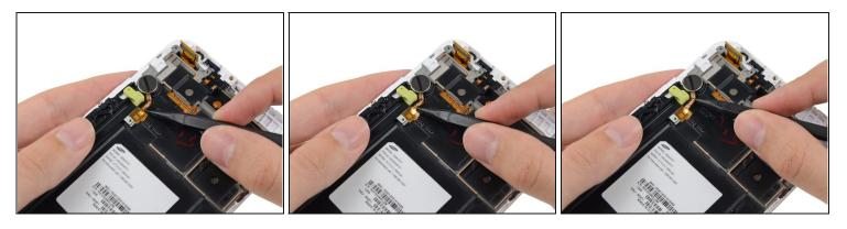
• Insert the tip of a spudger under the vibrator connector cable near the contacts then slide toward the vibrator itself.
