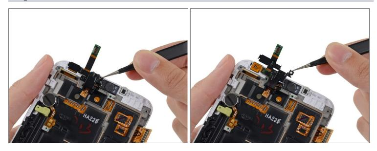
• Use a pair of <u>tweezers</u>, or your fingers, to remove the upper display assembly bracket.
