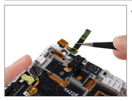
• Using tweezers, or your fingers, remove the front-facing camera assembly.
