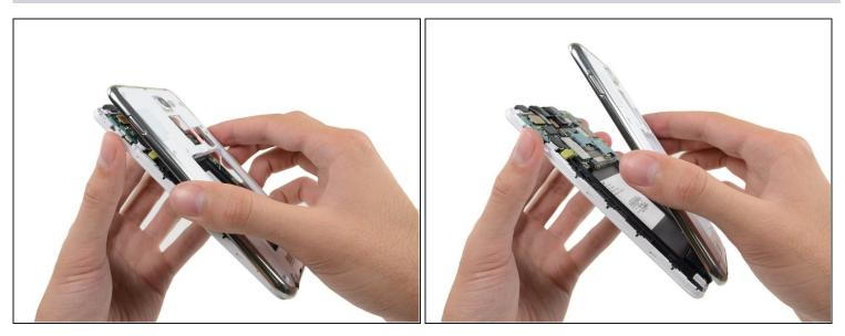
• Remove the midframe from the display assembly.
