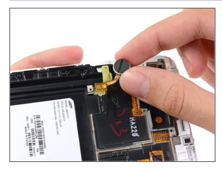
• Remove the vibrator from the display assembly.
