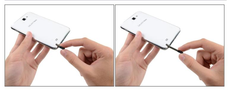
• Grasp the cap of the stylus and remove it from its slot in the midframe.
