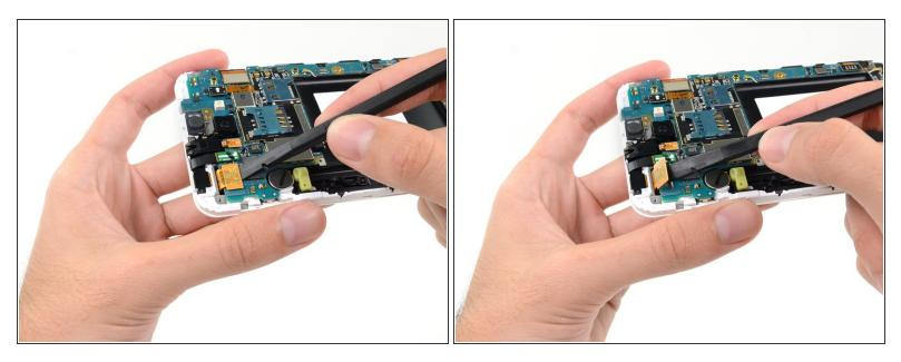
• Use the flat end of a spudger to carefully disconnect the display cable connector.
