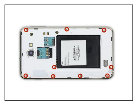
Remove the nine 3.4 mm Phillips #00 screws securing the midframe to the display assembly.
