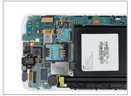
Remove the two 3.4 mm Phillips #00 screws securing the motherboard to the display assembly.
