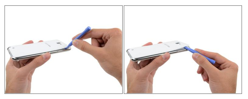
Pry with a plastic opening tool, or your fingernail, in the divot to the right of the rear-facing camera, near the volume rocker.
