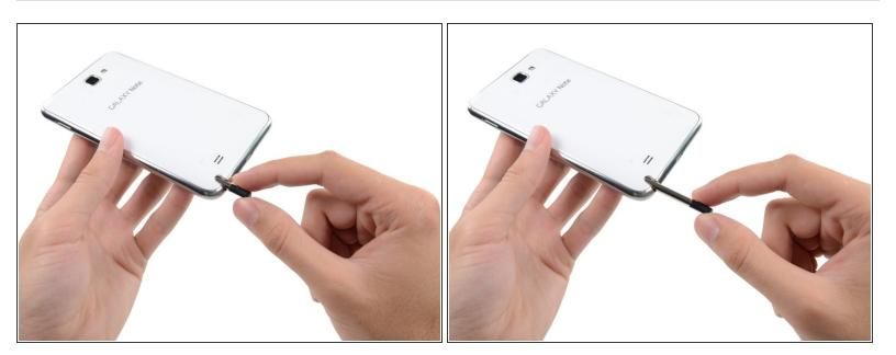
Grasp the cap of the stylus and remove it from its slot in the midframe.
