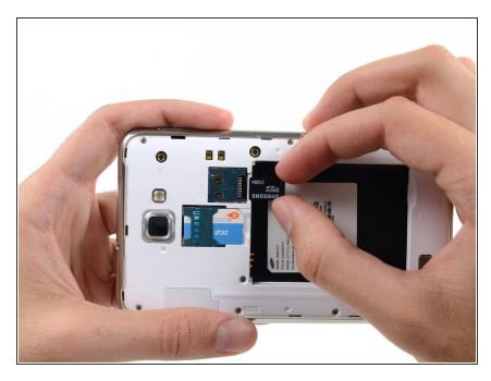
Remove the microSD card from its slot in the midframe.
