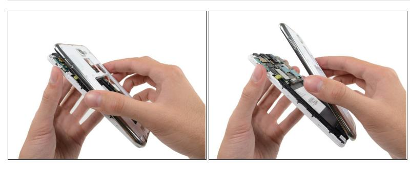
Remove the midframe from the display assembly.
