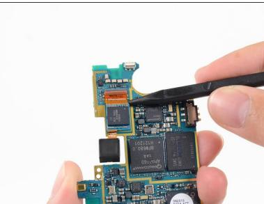
Slide the tip of a spudger under the rear-facing camera cable to slide it out of the ZIF connector and free it from the light adhesive.
