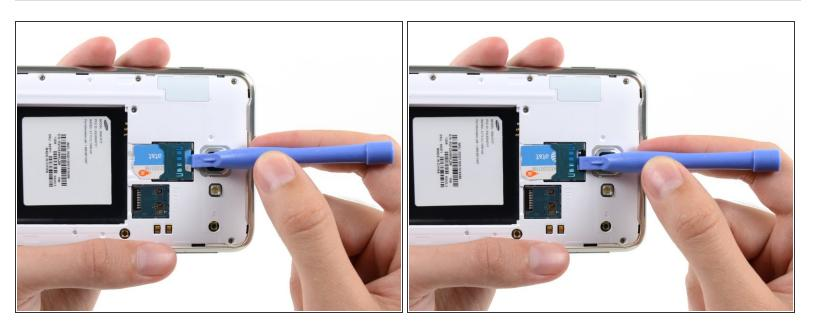
• Use a plastic opening tool, or your fingernail, to push the SIM card out of its compartment.
