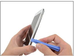
Slide the plastic opening tool down the seam.
