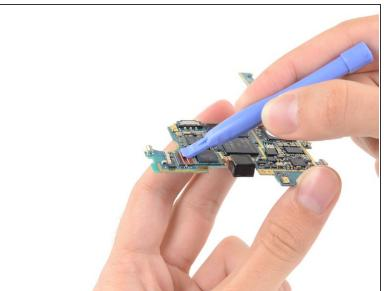
Use a plastic opening tool to flip the release tab on the rear-facing camera cable ZIF connector.
