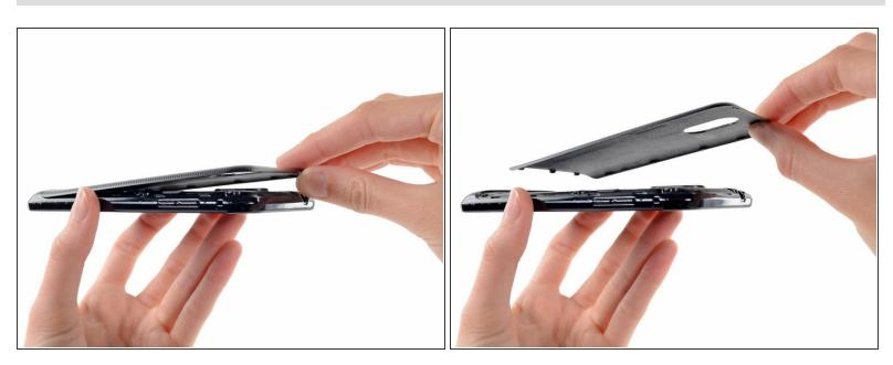
Lift and remove the rear case.
