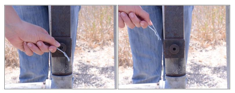
• Remove the two pins connecting the handle to the slider.
