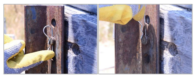
• Lift the two pins attaching the pump frame to the head and handle up, off of the pump frame.
