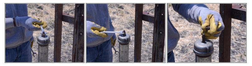
• Loosen and remove both the pump rod jam nut and pump rod nut on the top of the slider.
