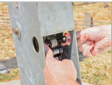
Remove the washer from the chain bolt.
