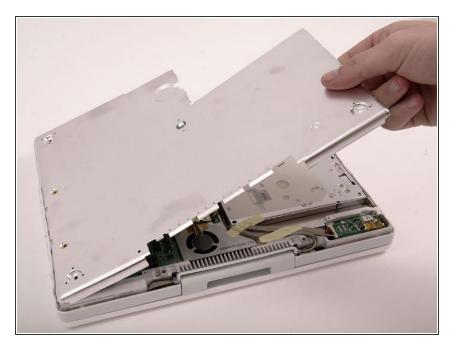
Lift the bottom shield off.
