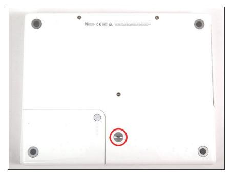
Use a coin to rotate the battery locking screw 90 degrees clockwise.
