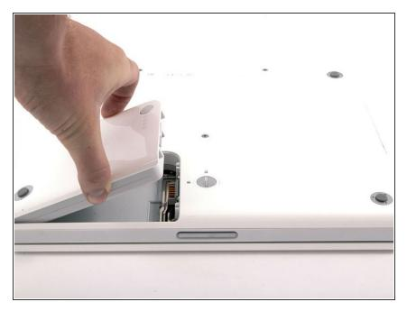
Lift the battery out of the computer.
