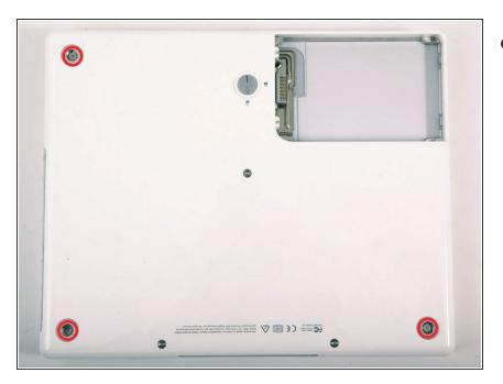
Remove the three newly-revealed Phillips screws.
