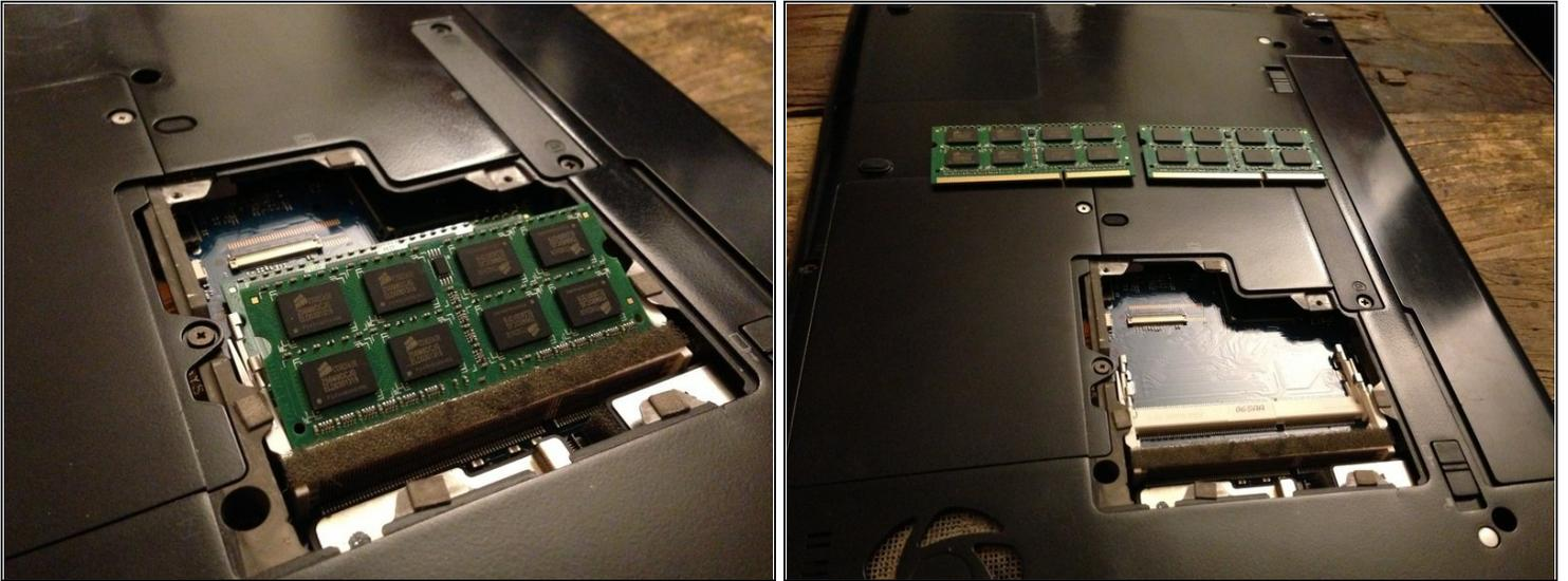
ⓘ After the tabs are popped off the RAM module, the module will rise and rest at a  $\sim 30^\circ$  angle. You can now correctly remove it.
