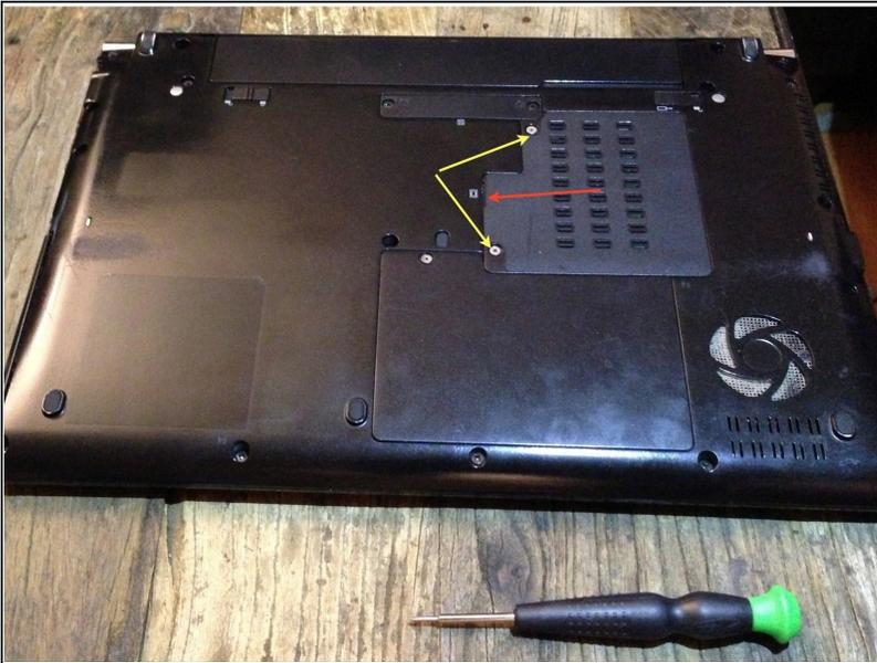
⚠ Fully power off the machine and remove the battery. Failure to do so may result in damage to the computer.
