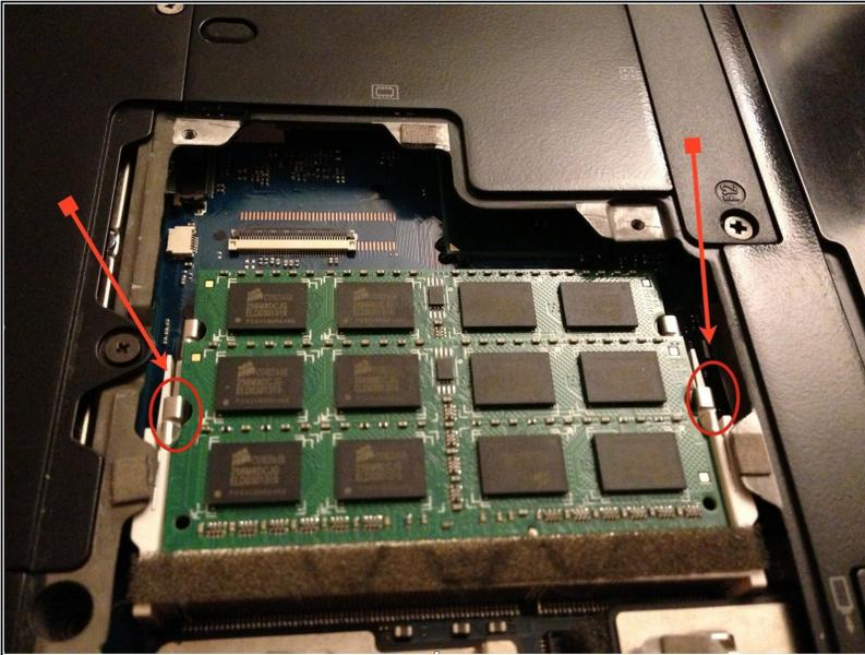
⚠ Ground yourself appropriately by touching a metal object outside your working space or by using an anti-static bracelet. Failure to do so may cause serious damage to your computer.
