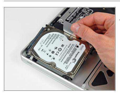
Lift the hard drive out of the upper case by its plastic pull tab, minding the cable attaching it to the computer.
