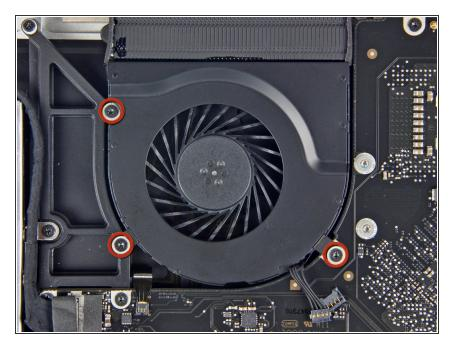
Remove the three identical T6 Torx screws securing the fan to the upper case.
