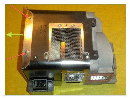
Remove both screws as shown and gently pull the metallic frame. It is anchored on two small notches on the other side.
