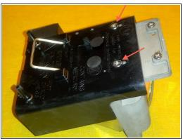
Remove the black stickers hiding both screws that will have to be removed in this step.
