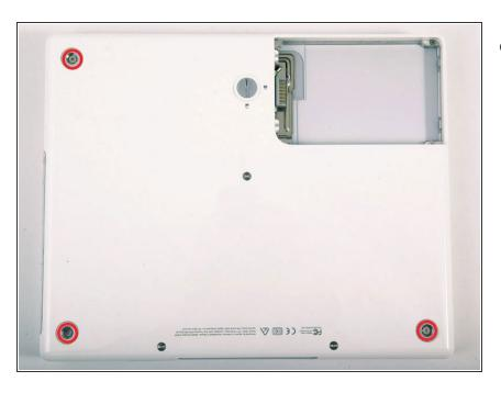
Remove the three newly-revealed Phillips screws.
