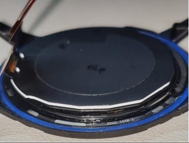
If the screen assembly gasket came loose during removal of the assembly, press it back into the groove on the underside of the screen assembly.
