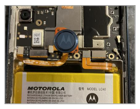
Disconnect the ribbon cables near the battery. Remove the 2 Phillips screws near the camera and near the top right corner.
