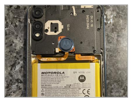
Unscrew the 21 Phillips #000 screws securing the top and bottom. There are screws under the S's. There is also one under the fingerprint reader. I was only able to take a picture of the top.
