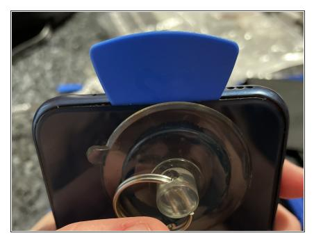
Quick, use a suction cup to rip off the adhesive! Put an iFixit opening pick to keep it open! Make sure to push the fingerprint sensor through while taking the adhesive off or you will rip the ribbon cable securing it.
