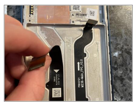
Peel off the cable securing the screen to the phone. Then heat the phone and use a suction cup to pull the screen away, make sure to pull the cable through the hole!
