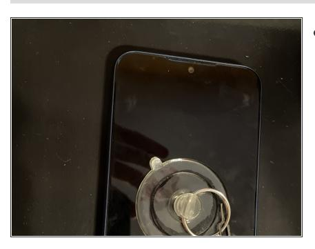
First, heat up the back of the phone using a heat gun, iOpener, or this heating mat I have. If you are using a heating mat like I am, I recommend putting a suction cup on the front so you can take it off the rubber surface. If you are using a heat gun or a heating mat, set it to 80°C (176°F) for 90 seconds.
