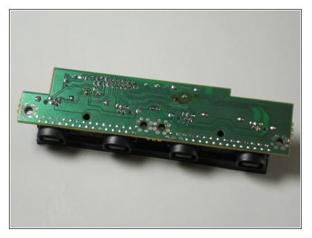
Flip the controller board on its underside so that the solder joints are exposed.
