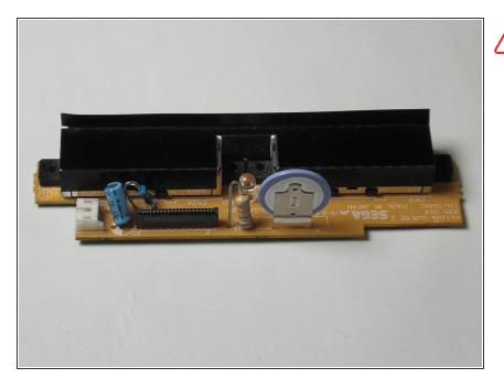
Verify that the resistor(s) leads do not touch other components on the topside of the circuit board. Otherwise, a <u>short circuit</u> may occur when you power on the system.
