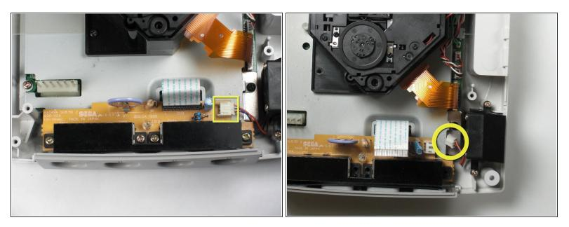
• **Disconnect the white fan header** from the controller port.
