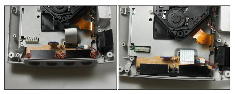
**Remove the four 14mm Philips #02 screws** located on the controller board.
