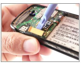
Use a plastic opening tool to gently pry the main motherboard cable connector away from the RAZR2.
