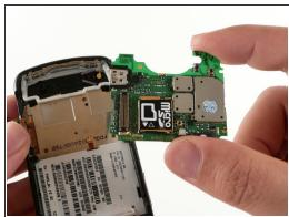
While holding the main motherboard cable connector away from the RAZR2, gently lift the motherboard away from the phone.
