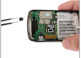
Use a pair of tweezers or your fingers to remove the small rubber cap from the motherboard.
