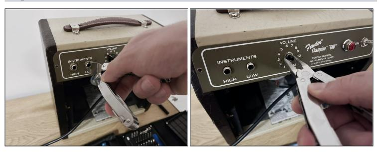
• Now it's time to remove the nuts on the input jacks and our broken volume pot - I used pliers to do that, but it is advisable to use a small adjustable wrench, combination wrench, or socket in order to avoid any unwanted scratches or damage.
