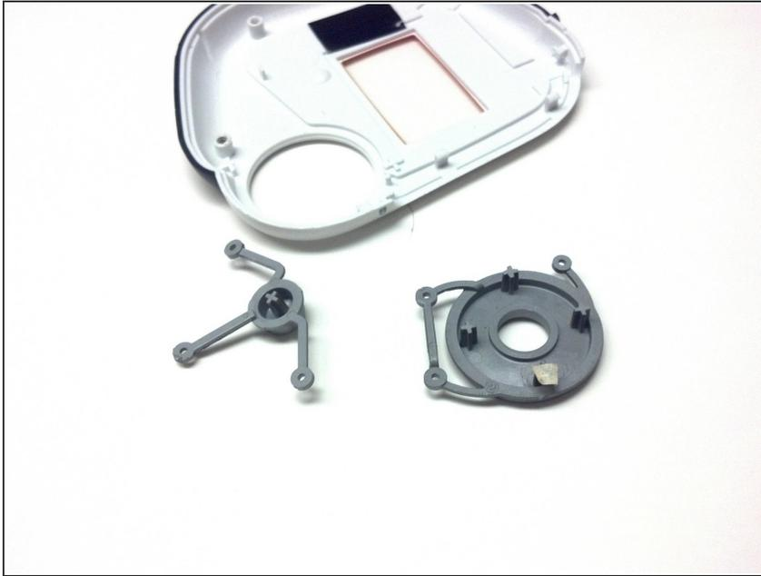
**⚠** All pins that hold the arms of the center button and the main plate of the face buttons have a slight flange at the top acting to hold the arm sockets. This is designed into the device at manufacture and removing the arm sockets will deteriorate the flange.
