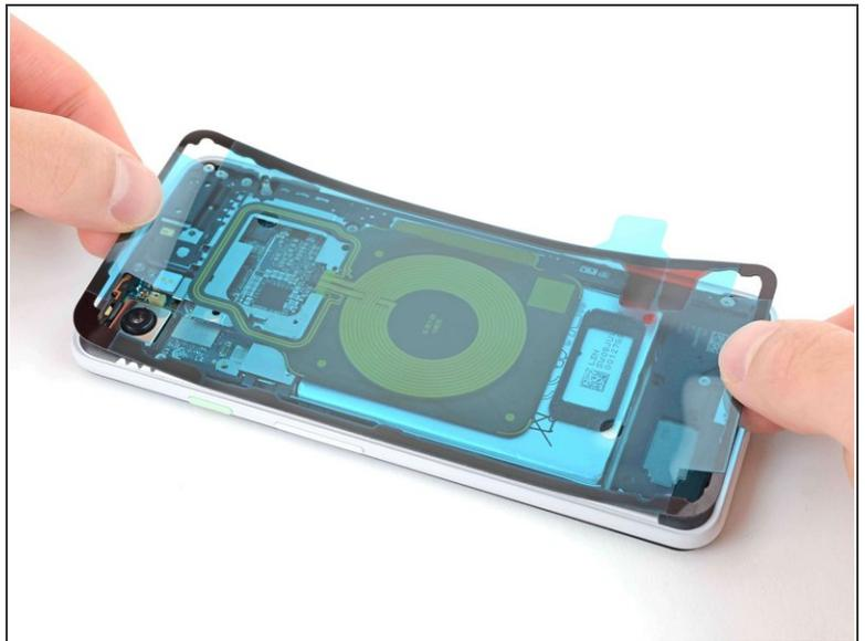
**⚠ Be very careful during this step! The adhesive is very sticky and can't be repositioned once it sticks. Misaligned adhesive can lead to an improper seal.**
