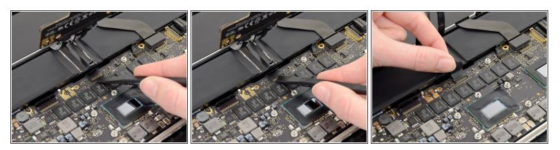
Repeat the previous procedure to disconnect the Trackpad ribbon cable from its socket on the logic board.
