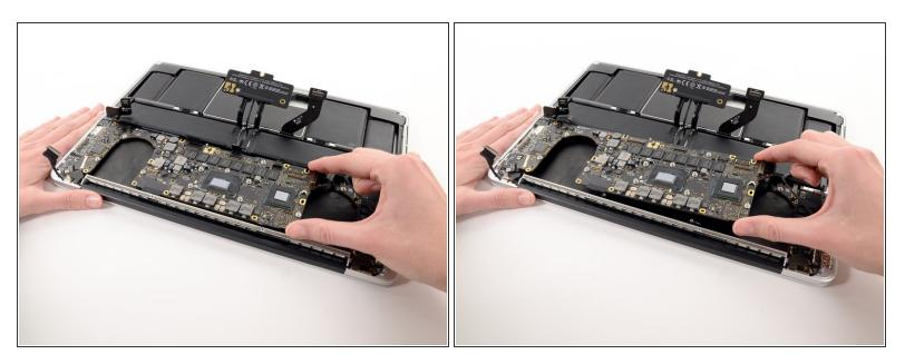
Carefully grasp the corner of the logic board (opposite of the I/O ports) and lift the logic board out
