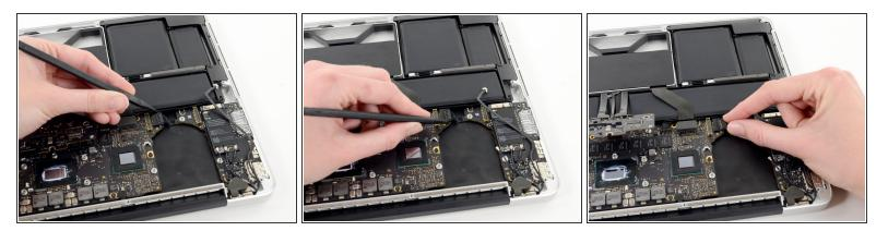
Use the tip of a spudger to push the edges of the I/O board connector straight out of its socket on the logic board.
