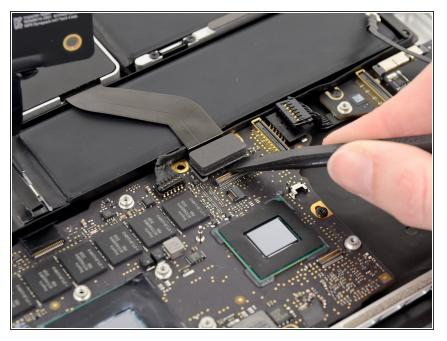
Use the flat end of a spudger to pry the SSD cable connector up off its socket on the logic board.
