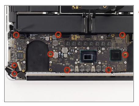
Remove the nine 3.3 mm T5 Torx screws securing the logic board and MagSafe DC-in board to the upper case.
