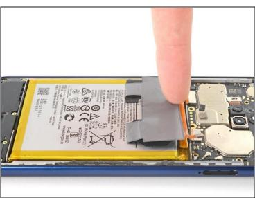
Fold the graphite heat dispersion film toward the top of the battery.
