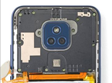
Use your Phillips screwdriver to remove the twelve 3.9 mm-long screws securing the motherboard cover.
