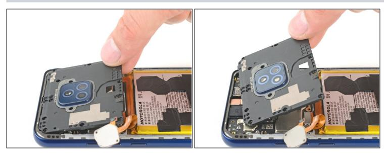
Grab the bottom edge of the motherboard cover and remove it from the frame.
