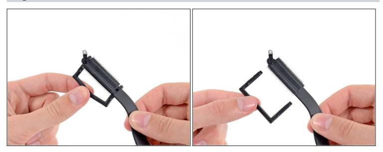
• Carefully remove the left fan duct from the edge of the heat sink.
