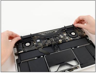
Lift and remove the heat sink up off the logic board assembly.
