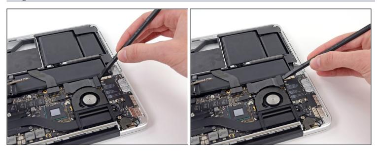
• Use the flat end of a spudger to pry the right side of the I/O board data cable connector up off its socket on the I/O board.
