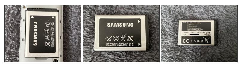
Inside the back cover we have an 3,7 Volts 800mAh Li-ion battery which is enough for a phone like that.
