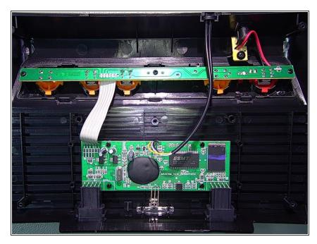
Unbox the bottom part by pushing laterally the plastic.
