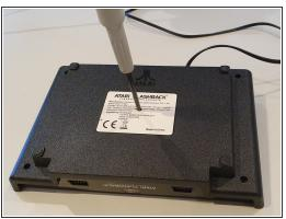
Un screw the 5 screws (Do not forget the one in the middle under the sticker).
