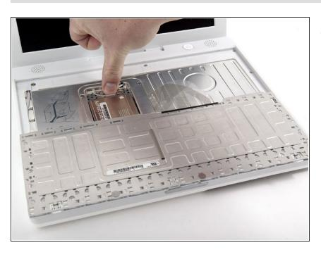
Push the wire clasp away from the AirPort card and toward the display, then rotate up to free it from the RAM shield.
