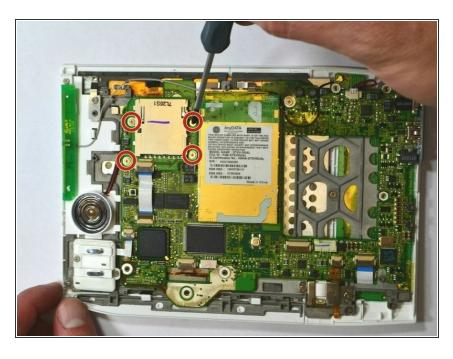
Remove the four (4) Phillips #00 screws (3 mm) which fasten the SD Card Reader.
