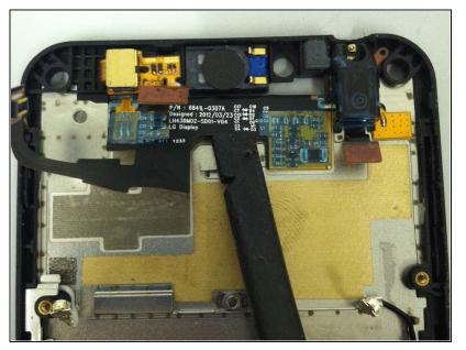
Peel off the adhesive portion of the LCD ribbon cable from the back of the phone
