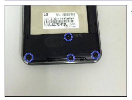
Remove the 4 Phillips 00 screws securing the speaker assembly to the phone housing.
