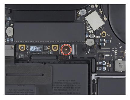
• Use a T5 Torx driver to remove the 3.7 mm pancake screw securing the battery power connector.
