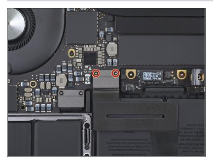
Use a T3 Torx driver to remove the two 1.8 mm screws securing the trackpad cable connector bracket.
