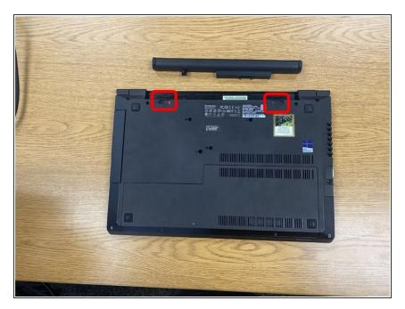
Move the switches to the unlocked position then push the battery out
