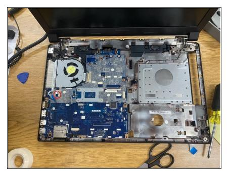
Remove the highlighted flex cable, then gently remove the cable and the LED.
