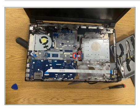
Disconnect the flex cable from the motherboard and then remove the two highlighted screws, and then pull it out.
