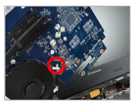
Pry the white nub out with a spudger to remove the charging cable.
