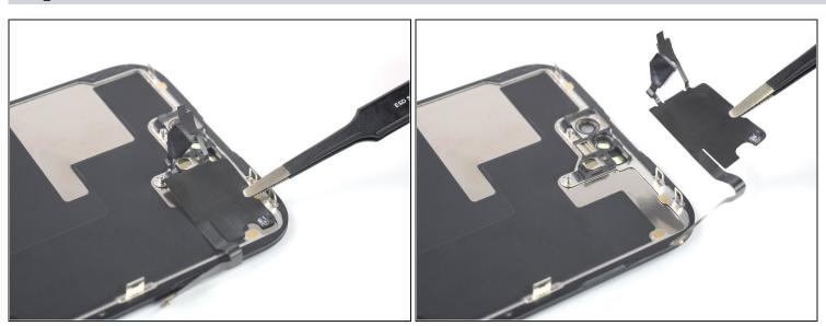
• Remove the front sensor assembly.
