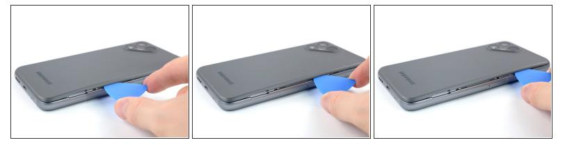
Using your thumbnail or an opening pick, slide along the right side of the phone to loosen the plastic clips.
