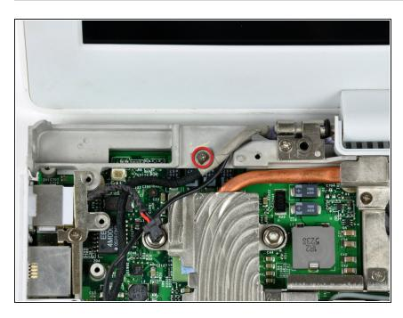
Peel up the yellow tape holding the display data cable to the metal framework and remove the single Phillips screw beneath it.
