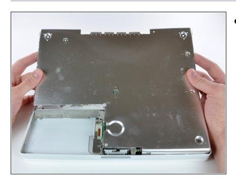
• Lift the bottom shield off.
