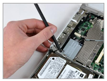
Using a spudger, pry up the AirPort/Bluetooth board from the end closest to the hard drive. Be sure to pry against the metal framework, as shown in the picture.
