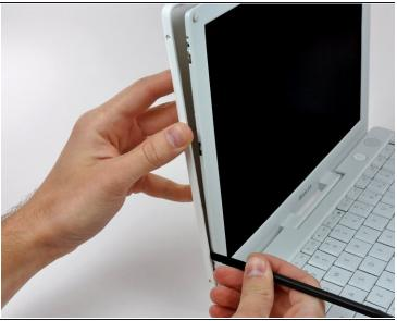
Working down from the upper left corner, use the flat end of a spudger to pry the rear bezel away from the left edge of the display.
