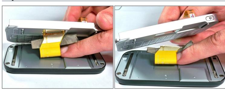
• Carefully pull the display cable through the opening in the keyboard panel. The keyboard panel can then be set aside.
