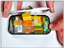
• Pry the silver cover off the screen enclosure. The display cable should be pulled through the opening in the silver cover.
