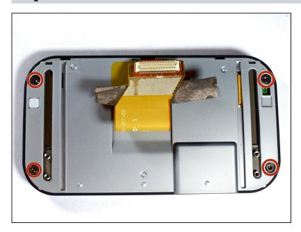
Remove four 5.0-mm Torx T6 screws from the screen enclosure.
