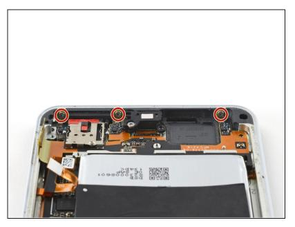
Use a T3 Torx screwdriver to remove the three 2.4 mm screws securing the charging assembly to the frame.
