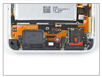
• Use a T3 Torx screwdriver to remove the 3.9 mm screw securing the USB-C port bracket to the frame.
