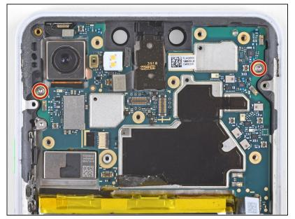
Remove the two 3 mm long T3 screws securing the motherboard.
