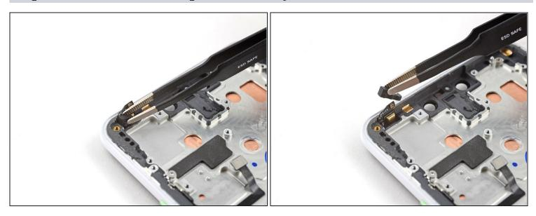
• Use tweezers to remove the rubber bracket between the microphone assembly and its recess in the frame.
