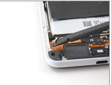
• Use the flat end of a spudger to pry up and disconnect the black coaxial cable connector from the charging assembly.
