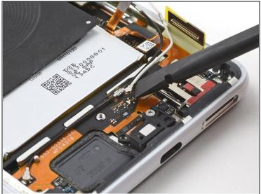
• Use the flat end of a spudger to pry up and disconnect the white coaxial cable connector from the charging assembly.
