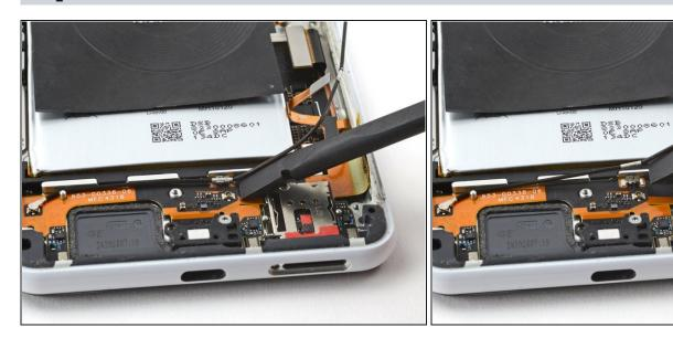
• Use the flat end of a spudger to pry up and detach the black coaxial cable from its clip on the charging assembly.
