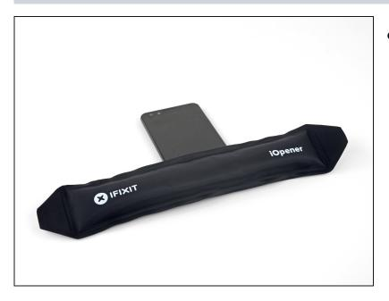
• <u>Heat an iOpener</u> and apply it to the bottom of the phone for one minute.
