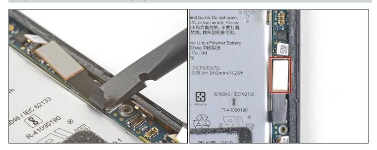
Use the flat end of a spudger to carefully pry up the black tape holding the display flex cable in place, near the right edge of the phone.
