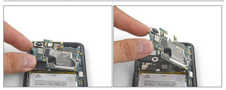
• Lift the left edge of the motherboard and carefully swing upwards it towards the right. Carefully push any press connectors snagging the motherboard out of the way.
