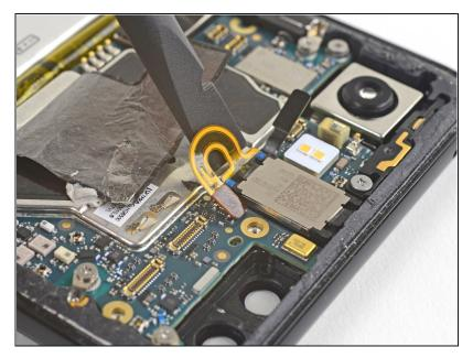
Use the flat of a spudger to carefully pry up and bend the earpiece speaker's flex cable upwards, out of the way of the motherboard.
