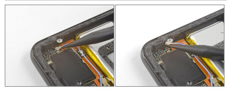
• Use the point of a spudger to pry up and disconnect the blue antenna cable from its socket on the charging assembly.
