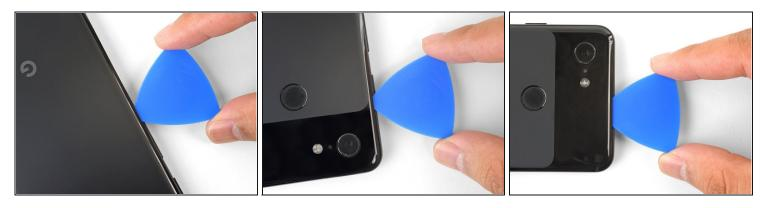
• Continue heating and slicing through the rest of the phone perimeter. Leave a pick in each edge to prevent the adhesive from resealing.
