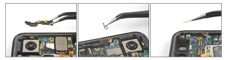
• Carefully remove the antenna bracket from the top left edge of the phone.
