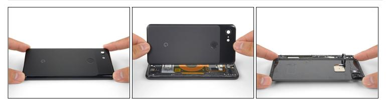
• Once you have sliced around the perimeter of the phone, carefully lift the **left edge** of the back cover.
