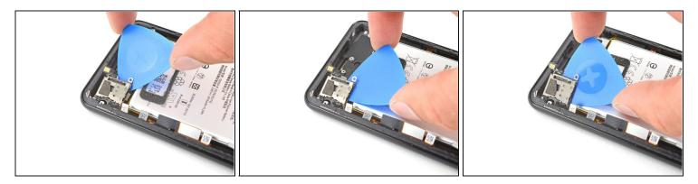
• Rotate the pick around the perimeter of the SIM card reader to separate the adhesive.
