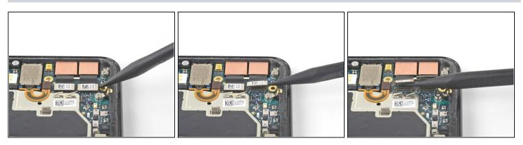
Use the point of a spudger to pry up and disconnect the connector for the camera(s) you are replacing.
