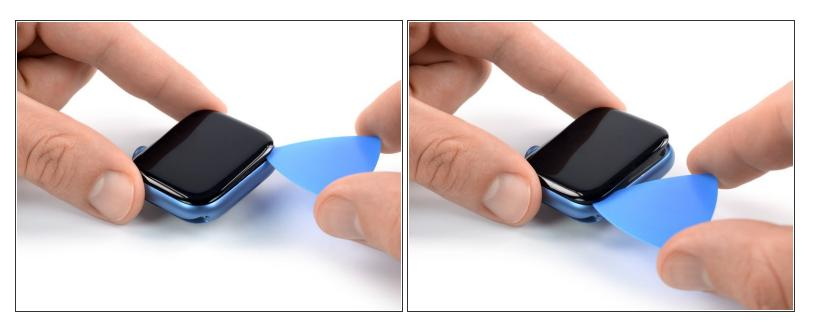
Slide the opening pick around the corner and along the long edge on the opposite side of the watch crown to slice the display adhesive.
