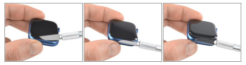
A Be aware that a sharp tool easily scratches your watch housing when not handled with care. To avoid undesired scratches, take your time and work carefully rather than hastily.
