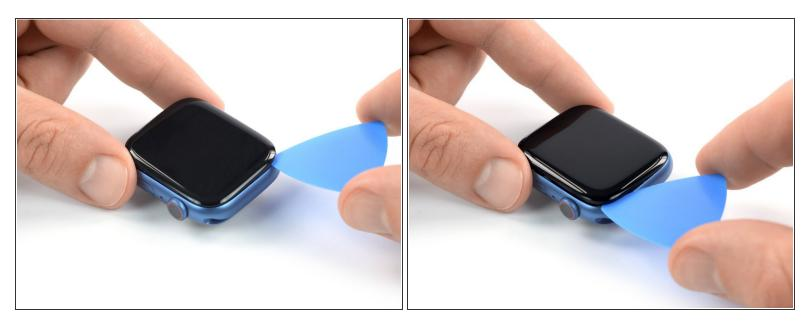
Slide the opening pick around the corner to slice the remaining adhesive on the short edge of the watch next to the watch crown.
