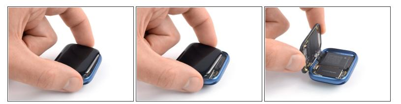
A Be careful not to strain the display cables when you fold the display to the side.
