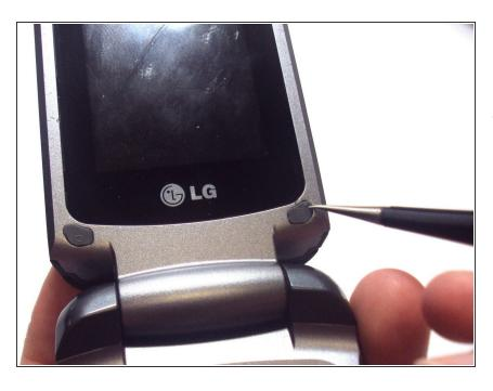
Use tweezers to remove the two rubber covers found at the left and right corners below the inside screen.
