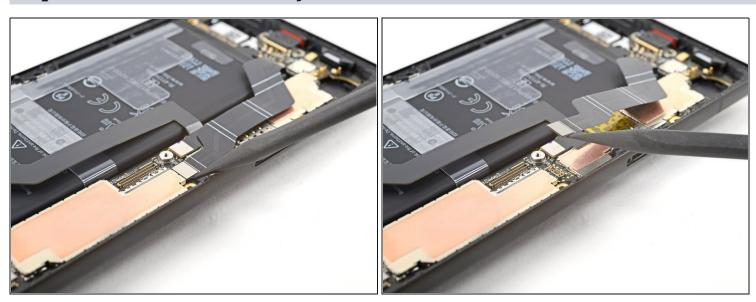
Use a spudger to pry up and disconnect the battery's press connector.
