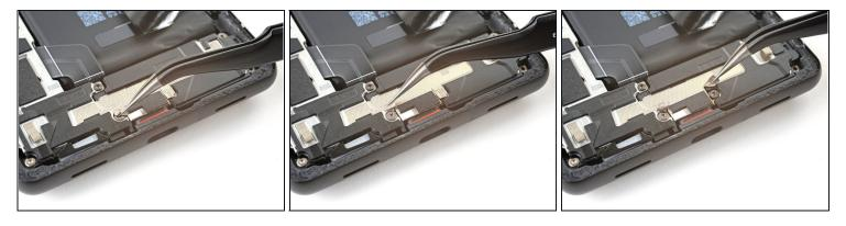
Use tweezers to peel back the tape covering the two screws on both sides of the USB-C port.
