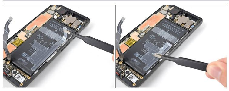
• Use tweezers, or your fingers, to peel the battery spacer away from the device.
