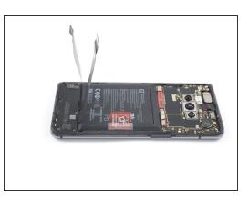
Bend the two flex cables toward the bottom of the phone and out of the way of the battery.
