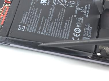
Use a spudger to carefully remove the adhesive tape on the left edge from the battery.
