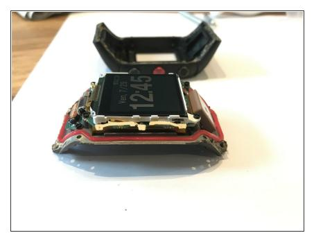
Disassemble the bracelet and open the watch (refer to the tutorial on replacing the motherboard <u>Polar</u> <u>V800 Motherboard Replacement</u>)
